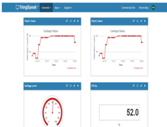
Figure 8: Web view of the person in charge when level is 52%
