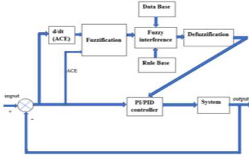
Figure 3. Schematic diagram showing the working processes of FGSPi and FGSPiD Controller
